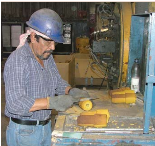
CORE FILES Blackhawk uses coldbox, nobake and shell cores in its castings.
