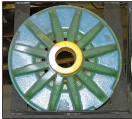
COLOR CODED The visual inspection area of the finishing department includes displays of typical castings (inset) that are marked with various colors to showcase areas in which defects may occur.
