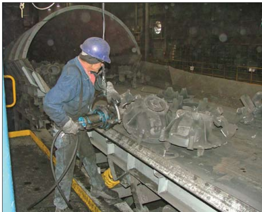
SAND WEDGE Pneumatic wedging devices are used to de-gate castings during shakeout.
